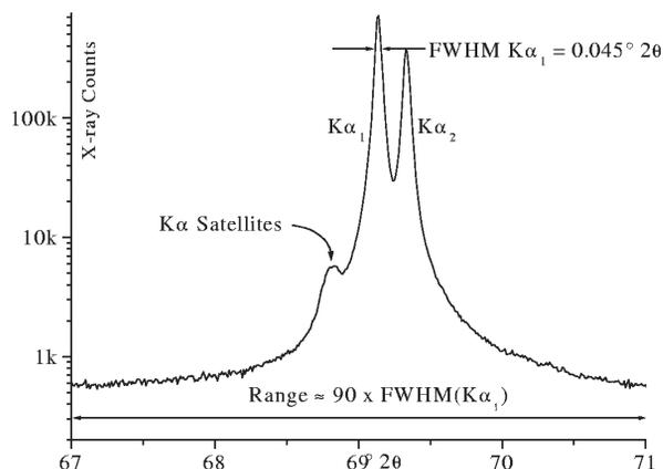
**Fig. 27.** Cu  $K\alpha$  emission profile showing the satellite group of lines and the extent of the tails from the  $K\alpha_1$  and  $K\alpha_2$  emission lines. This profile was recorded using the 400 line from a silicon single crystal wafer.
