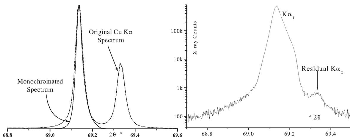
Fig. 29. Wavelength spectrum emerging from an asymmetrically cut Ge111 ground and bent incident beam monochromator presented linearly and logarithmically. The  $K\alpha$  satellites are completely removed, but the  $K\alpha_2$  is still present at  $\approx 0.02\%$  of  $K\alpha_1$  even in a well aligned system.
