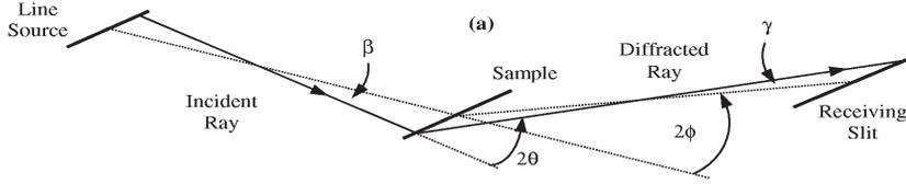
**Fig. 16.** An illustration of axial divergence in which the incident ray and diffracted ray are at angles of  $\beta$  and  $\gamma$  relative to the equatorial plane. Although the diffraction angle at the sample is  $2\theta$ , the diffracted beam is recorded at an angle  $2\phi$ .
