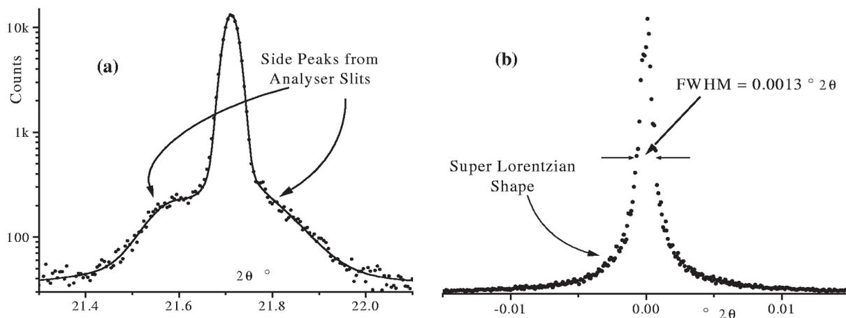
Fig. 9. (a) Reflection satellite peaks from analyser slit recorded using the 310 line from NIST standard material LaB<sub>6</sub> SRM 660a using the diffractometer on Station 2.3 at Daresbury synchrotron. (b)  $2\theta$  scan across a 0.1 mm  $\times$  0.1 mm incident beam using a Ge111 analyser crystal on beamline BM16 at the ESRF, Grenoble.
