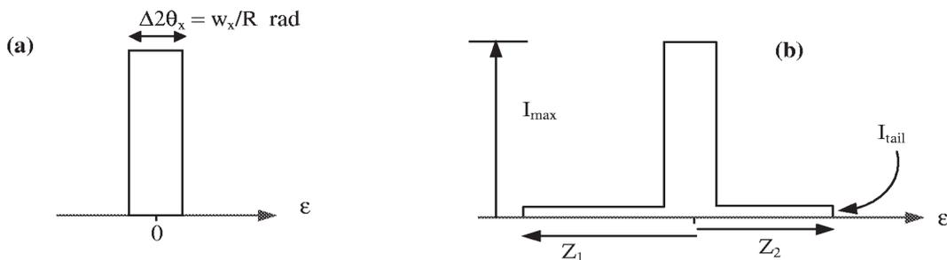
Fig. 6. Aberration profile models, (a) simple model for a source of projected width  $w_x$  and a diffractometer radius  $R$ , (b) model with “tube tails” containing additional parameters  $f = I_{tail}/I_{max}$  and angular widths  $Z_1$  and  $Z_2$  from the central maximum.
