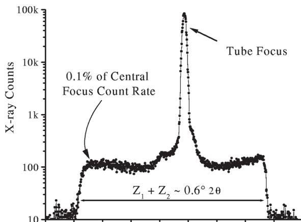
Fig. 7. Intensity scan with  $50 \mu\text{m}$  wide slit of an image formed through a  $10 \mu\text{m}$  pinhole in platinum of the  $0.4$  mm wide long fine focus in a Cu anode x-ray tube set at  $40$  kV,  $40$  mA.
