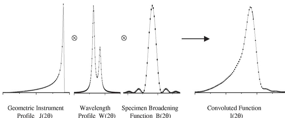
**Fig. 1.** Convolution of the geometric instrument profile  $J(2\theta)$ , the wavelength profile  $W(2\theta)$  and the specimen broadening function  $B(2\theta)$  to produce the measured convoluted function  $I(2\theta)$ .
