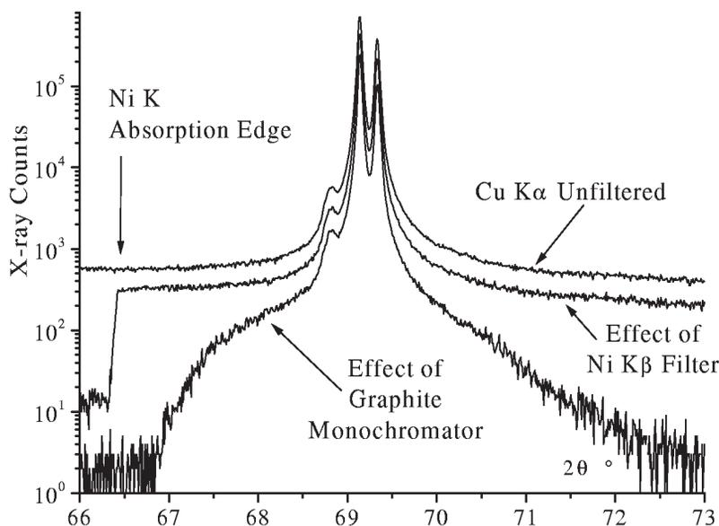
Fig. 28. Cu  $K\alpha$  emission profile obtained using the 400 line from a silicon single crystal wafer. Each pattern was recorded sequentially using the same sample, first with no filter or monochromator in the beamline, then with a Ni  $K\beta$  filter, and finally with a standard curved graphite diffracted beam monochromator.
