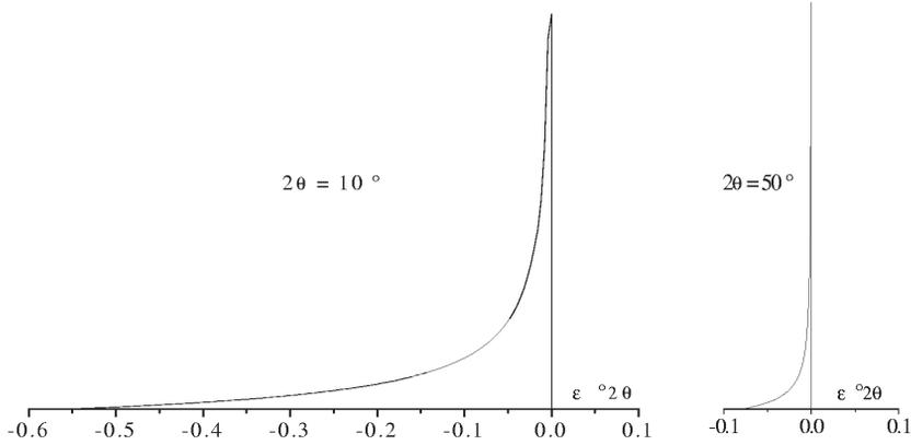
**Fig. 18.** Axial divergence aberration profiles  $J_{AX}(\epsilon)$  for a diffractometer with no axial divergence in the incident beam. This was calculated using Eq. (17) for  $L_S = 10$  mm,  $L_R = 15$  mm, and  $R = 215$  mm at  $2\theta = 10^\circ$  and  $2\theta = 50^\circ$ . A very narrow Lorentzian profile was convoluted with  $J_{AX}(\epsilon)$  to overcome the infinities at  $\epsilon = 0$ .
