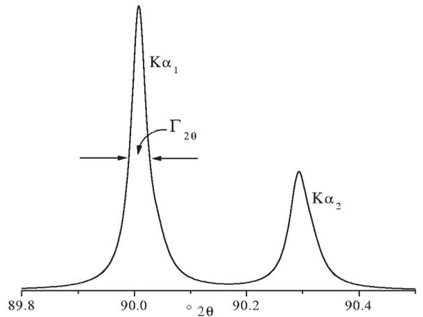
Fig. 24.  $K\alpha_1\alpha_2$  emission profile from copper recorded using the 400 line from a silicon single crystal.
