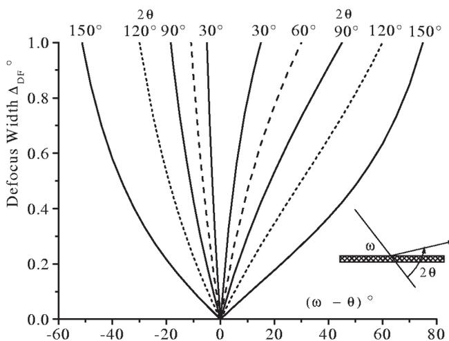
Fig. 15. The variation of defocussing width  $\Delta_{DF}$  with  $(\omega - \theta)$  at different  $2\theta$  diffraction angles.
