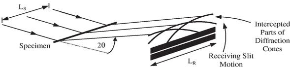
**Fig. 17.** Arcs formed in the vicinity of the receiving slit by the diffraction cones radiating from all points across the sample axis. The axial divergence aberration function is the profile shape detected by an infinitely narrow receiving slit as it scans through the arcs.
