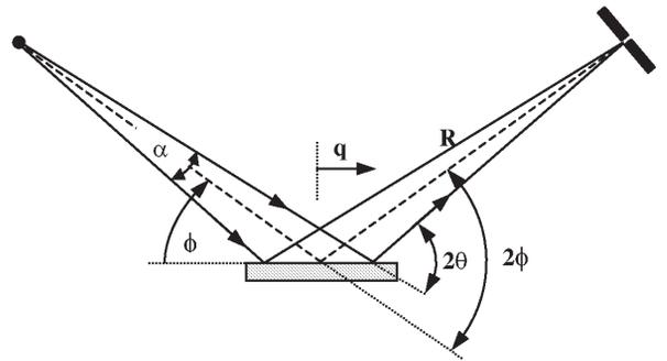
Fig. 11. Diffraction from a flat plate showing the relationship between the measured angle  $2\phi$  on the diffractometer and the diffraction angle  $2\theta$  for a ray at the outer limit of a beam of divergence  $\alpha$ .
