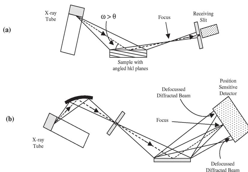
**Fig. 4.** (a) Diverging beam diffractometer operated in asymmetric mode with defocussed diffracted beam at the receiving slit, (b) diffractometer with PSD replacing the receiving slit. Diffracted beam is in focus at the centre of the detector and defocussed in off-centre positions.
