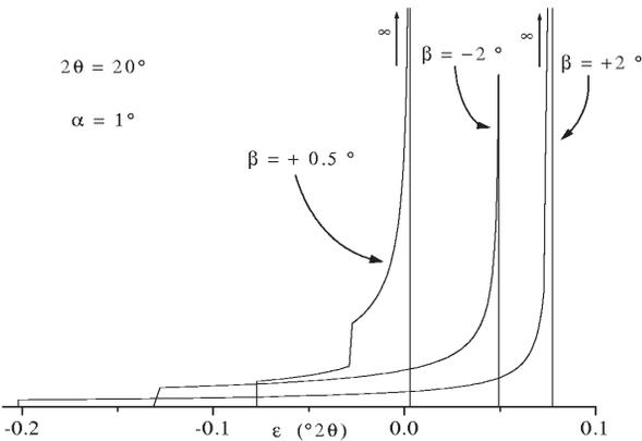
Fig. 22. LPSD flat specimen error/defocussing aberration function  $J_{\text{PSD}}(\varepsilon)$  for an incident beam of divergence  $\alpha = 1^\circ$  at  $2\theta = 20^\circ$ . Examples are given of  $J_{\text{PSD}}(\varepsilon)$  near the centre of the PSD ( $\beta = 0.5^\circ$ ) and at  $2^\circ$  either side of centre (ie.,  $\beta = +2^\circ$  and  $-2^\circ$ ).
