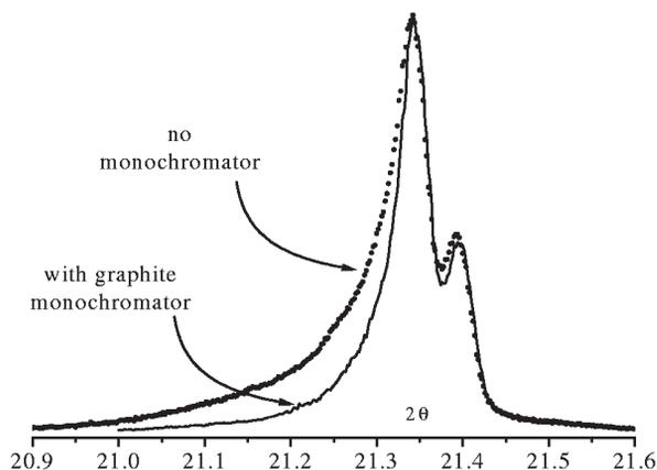
**Fig. 20.** Effect on the 100 profile from  $LaB_6$  powder of including a graphite monochromator in the diffracted beam in a diffractometer with no diffracted beam Soller slits. The two profiles were normalised to the same peak intensity  $I_{max}$ .
