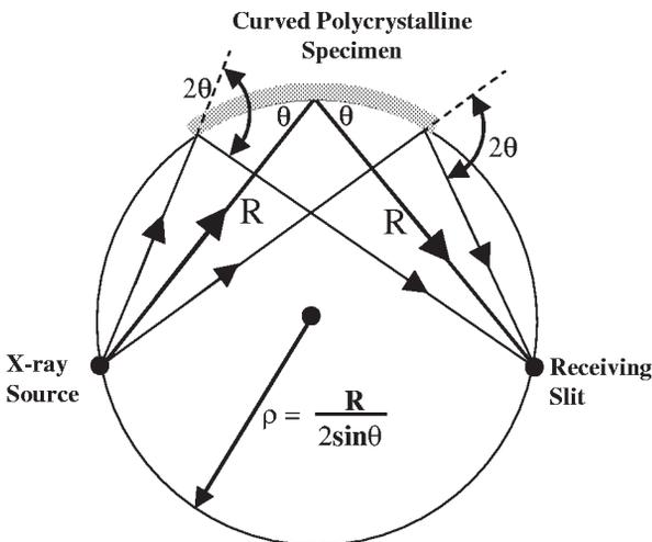
Fig. 10. Focussing in a symmetric powder diffractometer.
